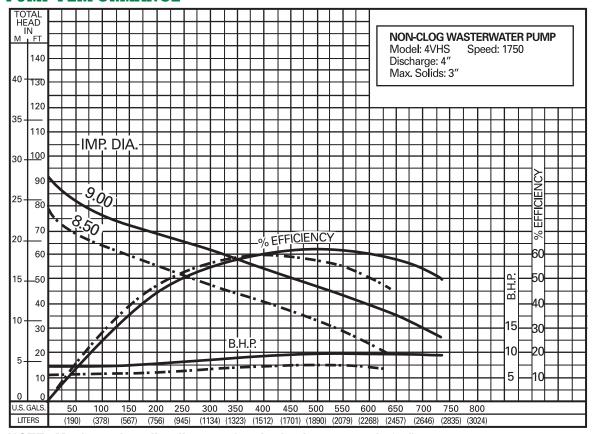
NOTE: Maximum impeller diameter for single phase pump is 8.5"
