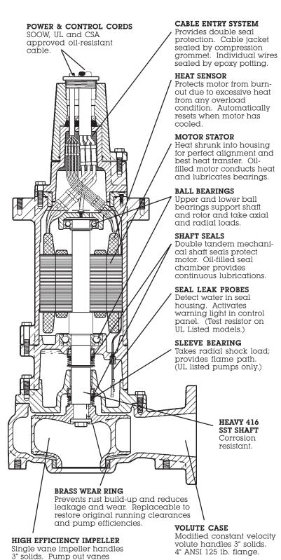
help keep trash from seal; reduces pressure at seal
