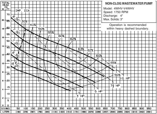
Pump performance is based on clear water (1.0 specific gravity @ 68°F) and pump fluid end (hydraulic) efficiency. Motor data based on 40°C ambient temperature.
