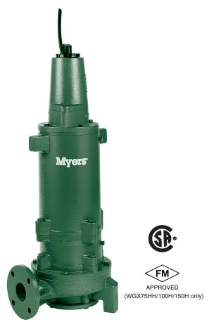
YERS HIGH HEAD 7½, 10 & 15 HORSEPOWER SUBMERSIBLE CENTRIFUGAL GRINDER PUMPS ARE DESIGNED FOR MUNICIPAL, COMMERCIAL OR INDUSTRIAL APPLICATIONS. These pumps are especially suited for use in pressure sewer applications or in systems with long discharge runs or high static heads. The pumps feature a heavy-duty cutter mechanism and recessed impeller designed to efficiently grind typical sewage solids into a fine slurry.
