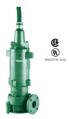
THE MYERS WG30-50 ARE RUGGED 3-5 HORSEPOWER SUBMERSIBLE CENTRIFUGAL GRINDER PUMPS DESIGNED FOR RESIDENTIAL, LIGHT COMMERCIAL, INDUSTRIAL OR MUNICIPAL APPLICATIONS. They are especially designed for grinder pump applications requiring higher flows at low to moderate heads. The WG30-50 feature a heavy-duty cutter mechanism and recessed impeller design to efficiently grind typical sewage solids into a fine slurry.
