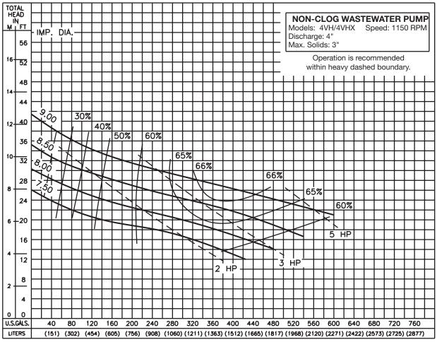
Pump performance is based on clear water (1.0 specific gravity @ 68°F) and pump fluid end (hydraulic) efficiency. Motor data based on 40°C ambient temperature.
