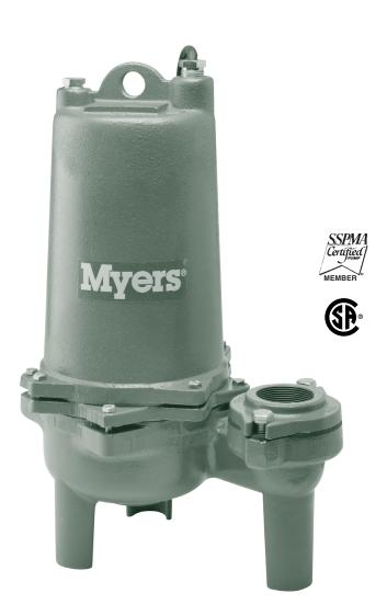
THE WHR5H-WHR20H SERIES PUMPS ARE DESIGNED FOR USE IN LIGHT COMMERCIAL AND RESIDENTIAL RAW SEWAGE AND EFFLUENT APPLICATIONS. They deliver higher heads than standard sewage pumps and will pass 2 inch solids. Recessed vortex impeller provides an unobstructed passage in the volute case, allowing the pump to handle stringy trash without plugging the impeller. For more information, call your Myers distributor, or the Myers Ohio sales office at 419-289-6898.
